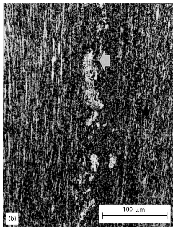
Figure 10 Optical micrographs of welding interface of the multiple upset welded copper wires at various preheating temperatures. (a) As hot rolled, (b) 673 K, (c) 773 K, (d) 873 K, (e) 973 K and (f) 1073 K.
